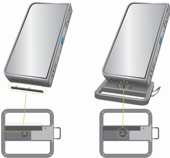
To set up the codec vertically on its base, remove the cover on the left side of the Codec Unit and insert it into its base. Fully turn the connecting screw on the base, and make sure it is completely secured.
